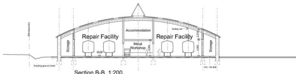
Section B-B 1:200 The Repair Facility
